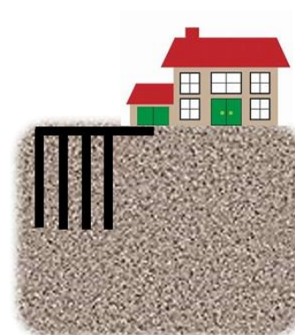
Figure 1-3: Thermally interacting boreholes - BTES
