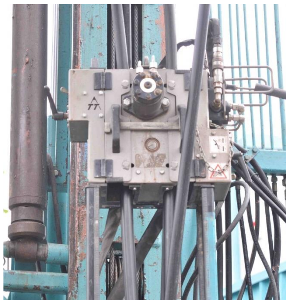
Figure 2-14: Detailed view on the pipe drive
