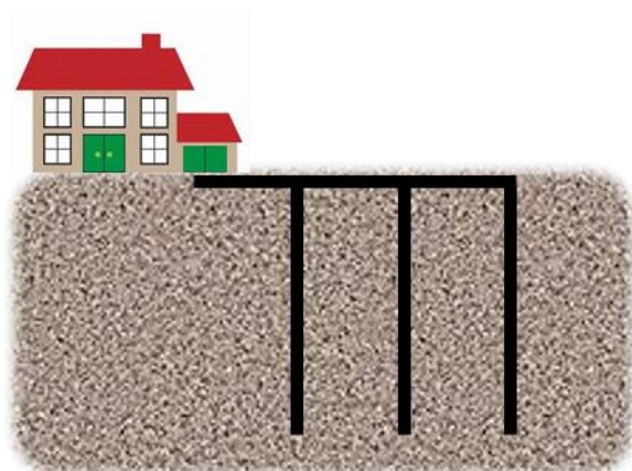
Figure 1-4: Independent boreholes - GSHPs
