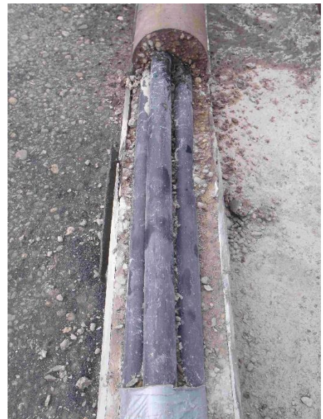
Figure 2-18: Vertical section of a grouted borehole
