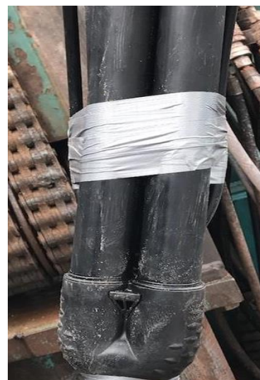
Figure 2-10: The down end of a single U pipe
