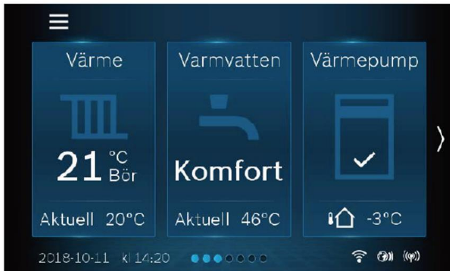
Figure 3-34: An example of display for monitoring and control in the smartphone application [9]
