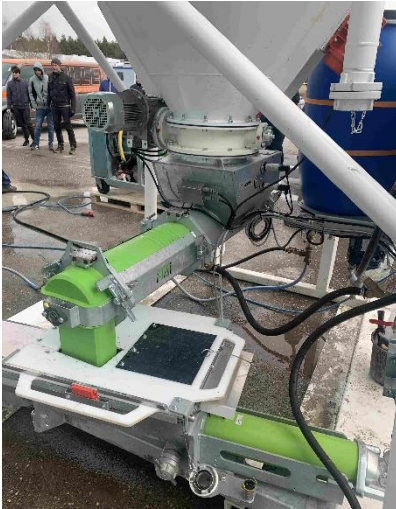
Figure 2-17: Continuous mixer with screw pump for high pressure grouting
