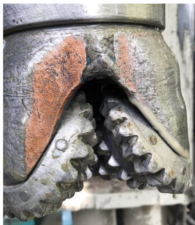
Figure 2-5: Tricone drill bit
